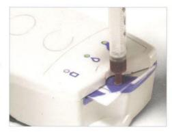
epoc test cards are single-use bar code identified units containing a biosensor array, calibration solution and fluidics. Test cards generate electrochemical assay signals and quality control signals which are read by detectors in the epoc Reader.
